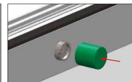
Screw on outer sleeve
