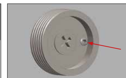
Secure with 3mm grub screw
