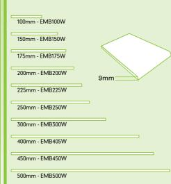
9mm thick Soffit Board (Multi-Purpose Board) is designed to close the gap between the edge of the fascia and the brick work. 9mm 'Core' Soffit is available in 11 lengths.
